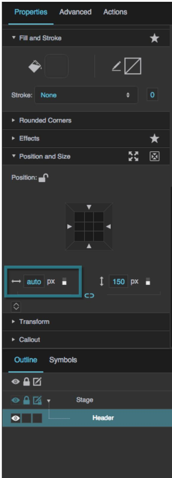
Because the Stage's **Horizontal Alignment** is set to **Stretch**, the header's width of **Auto** makes the header expand to follow the size of the Stage.
